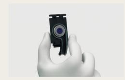
I Condensate outlet undamaged. Gaskets (housing and bellows) intact.
