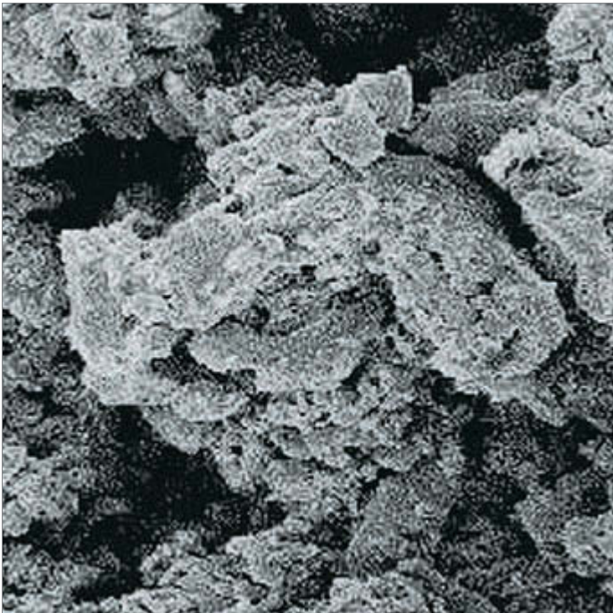
Plasmapore XP® innovative surface technology made of porous titanium for enhanced stability
